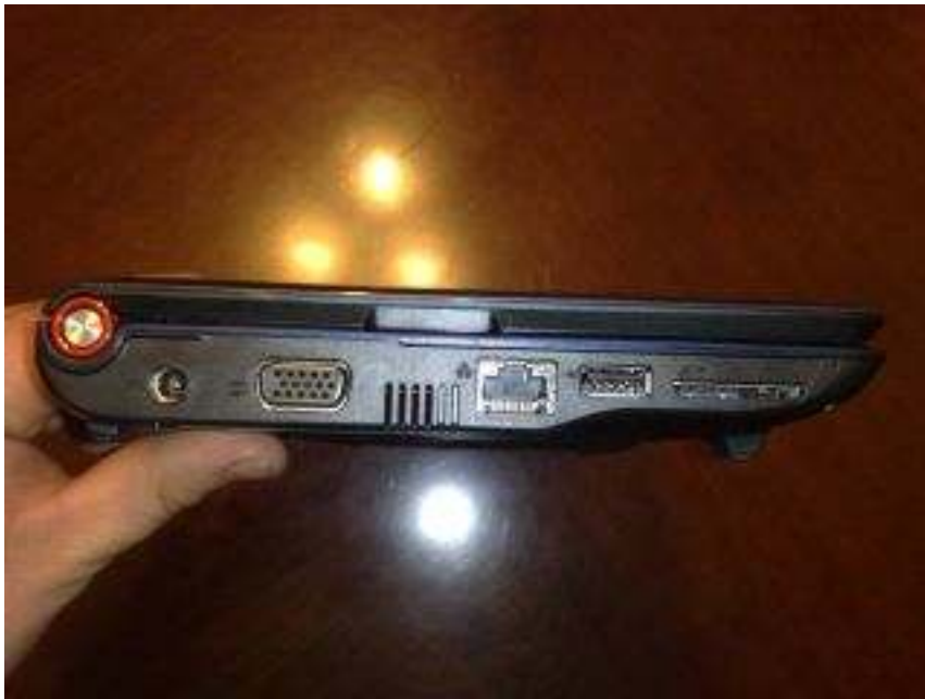
Ports from left to right - AC Power In, D-Sub Out, Output Fan, Ethernet port, 1 x USB 2.0 port and a SD Storage Expansion slot.
