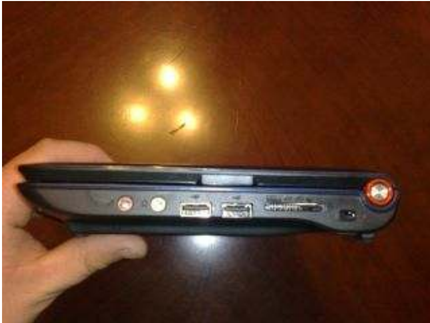
And on the right hand side of the unit we have (from left to right) - Mic In, Audio Out, 2 x USB 2.0 ports, Multi-In-1 Card reader and a Kensington lock slot.
